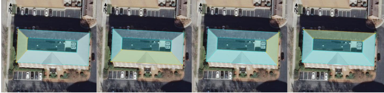
Figure 53. Using the snapping tool to build a roof structure by sections.
