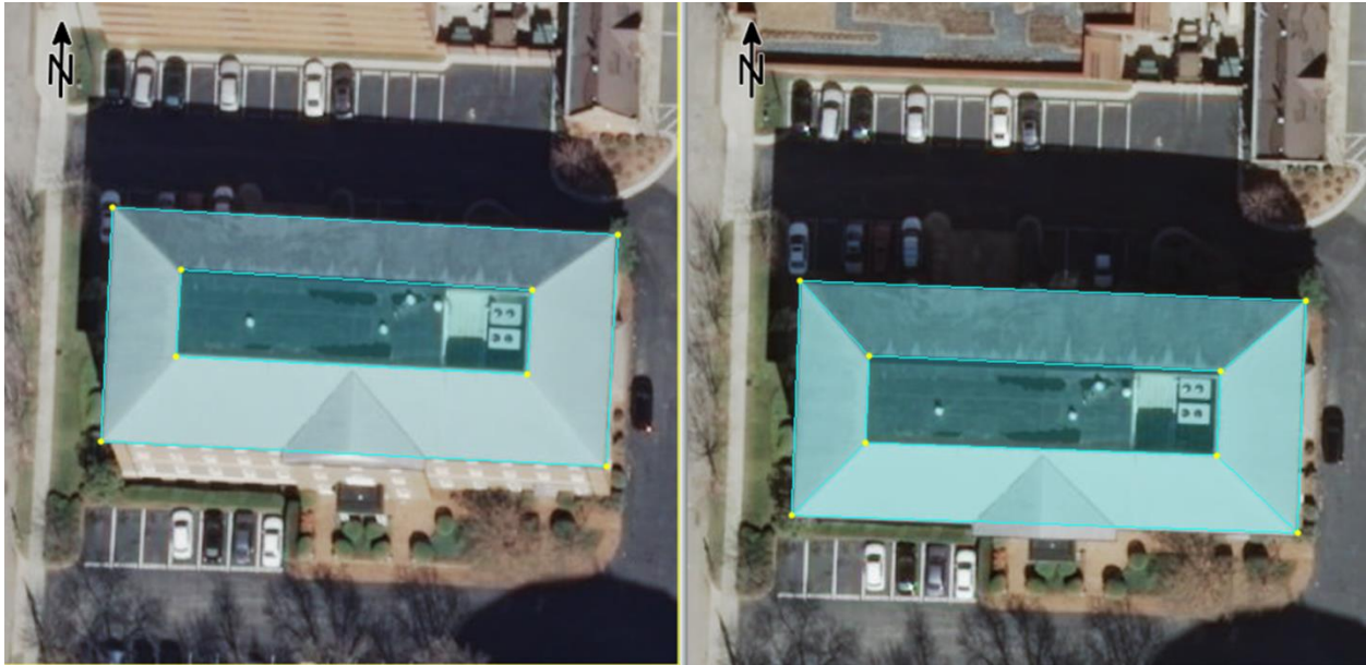
Figure 52. Loft a polygon to another polygon to create a truncated pyramid.
